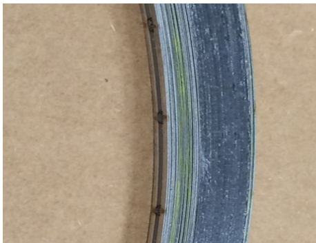
Figure 2. The figure above shows the increased spot welds as well as the multiple layers of interior metal windings which act as an inner ring.
